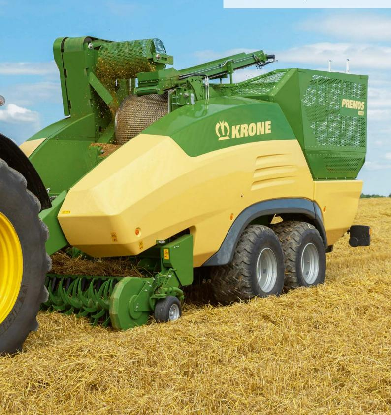
The mobile pellet harvester and stationary mill
